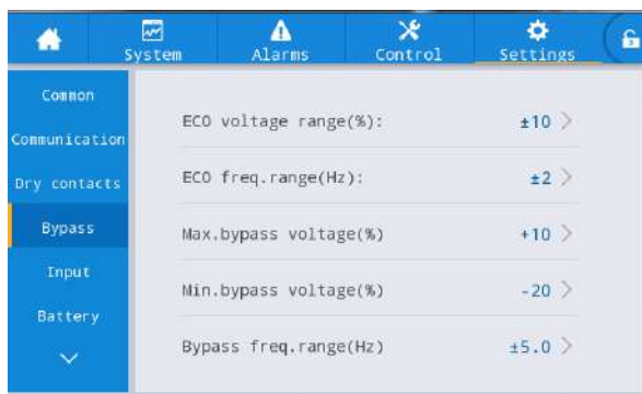
Fig. 4-22 Bypass parameters interface
