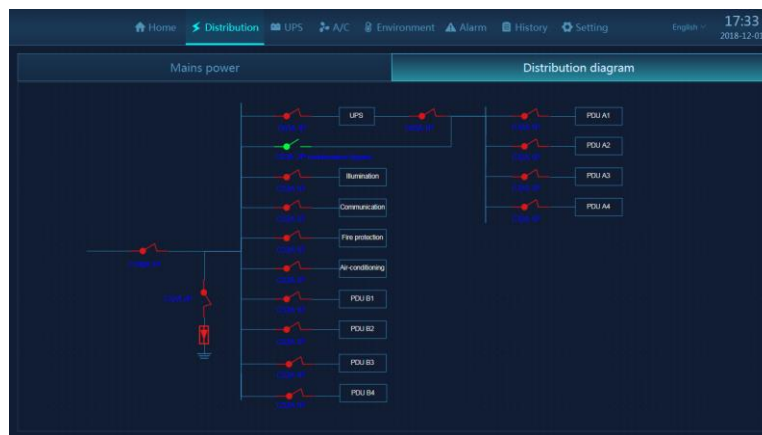
Fig. 4-6 Power distribution - power distribution interface)
