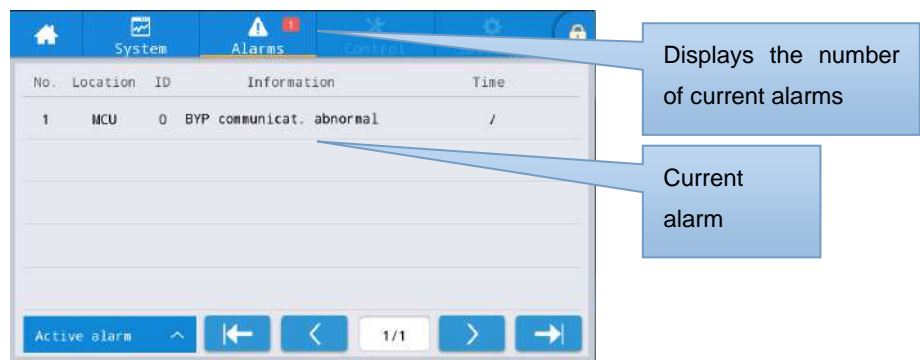
Fig. 3-16 Current alarm interface
